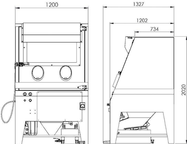
Fitted with the Vapormatt MK3 10mm Blast gun, air blow-off nozzle and a recirculated water system with a diaphragm pump.
