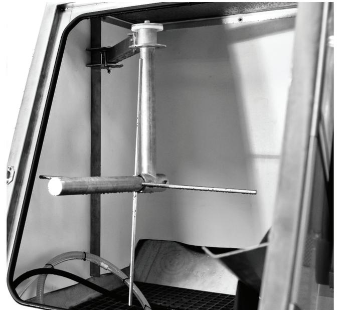
A front loading swing door (with safety lock) allows the operator easy access to the swing arm jig to assist with loading and unloading, the jig features a 48mm shaft over which a wheel can be located, the back of the wheel rests up against x4 round bars and is free to rotate around the central shaft which inclines backwards.
