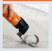
New flooring needs a clean surface. The stopper knife allows you to remove even stubborn residue left behind by old floor coverings.
