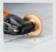
For continuous use, the diamond or carbide-coated saw blades are also available as a round version. These 360° coated tools can rotate 3–4 times and thereby have a longer service life than segmented blades.
