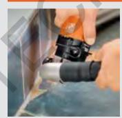
The extraction device and diamond or carbide-coated tool can remove tile joints economically and precisely while producing very little dust.
