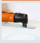
With the FEIN cutting tool, the channel for hot water underfloor heating is cut directly in the panel.
