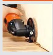
The HSS saw blade for wood is excellently suited to accurate sawing e.g. parquet or laminate flooring. Fired stoves can therefore be subsequently fitted with ease, and working with wall and ceiling coverings is child's play.
