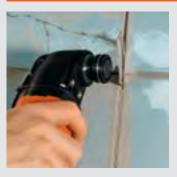
Excellently suited to cutting out particularly hard tile joints such as extremely waterproof epoxy resin joints in swimming pools.
