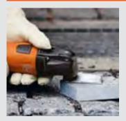
The cleaning block is used to re-sharpen and clean diamond tools, enabling you to remove sealant residue and other impurities at speed and with ease.
