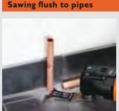
Copper heating pipes which are no longer needed can be sawn off flush to the wall or floor using the stepped E-CUT universal saw blades – even in hard-to-reach places.
