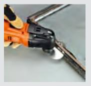
The mushroom-shaped cutter blade cuts insulation windows at speed and with ease. Undamaged single panes can be used for repairs elsewhere. Separating materials for disposal is extremely easy.
