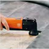
The carbide rasp can remove plaster and screed residue or sand down tile adhesive before re-tiling at speed and with ease.
