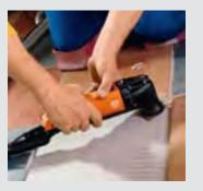
Even thick layers of tile adhesive can be easily ground away when replacing individual tiles. Dust extraction, suitable for the FSC 2.0 Q corded machine, avoids dirt and dust.
